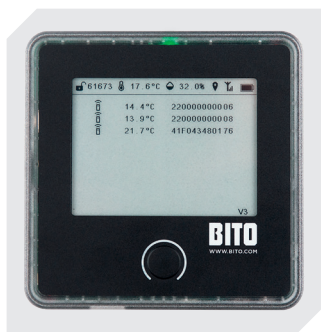
SmartHub Gateway monitoring system L 129 x W 129 x H 29 mm 77-51269
