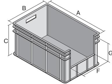
Pos. Dimensions, tolerances as specified in DIN 16901
