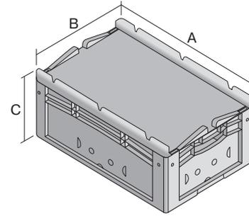
Pos. Dimensions, tolerances as specified in DIN 16901
